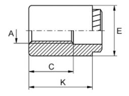
Female thread A = M2,5 Height K = 12 Hole diameter +0.1 = 4.2 Min distance to edge = 2.4 Min material thickness = 1.5 Outer diameter E = 6 Thread length = 9
